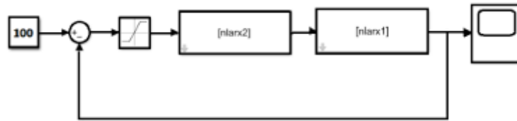
Fig. 10. Inverse approach of CL control system for glucose regulation using NLARX models
