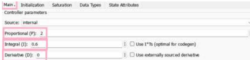
Fig. 8. Adjusting the PID controller main values settings
