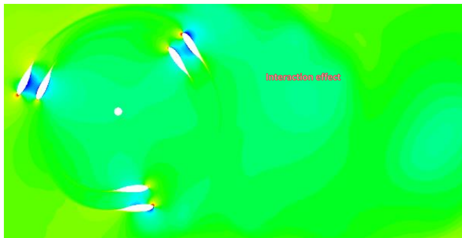
Figure 3.22. Total pressure contour of Design-2 for Uniform WSP.
