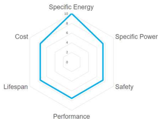
Fig. 4. Characteristics of NMC or Lithium Nickel Manganese Cobalt Oxide ( \text{LiNiMnCoO}_2 ) Battery (Blackridge Research 2025)
