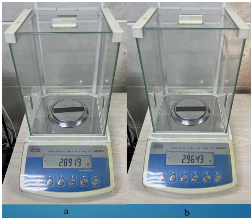
Figure 4. a: Initial weight of the flexure specimen; b: Weight measurement after 10 days.
