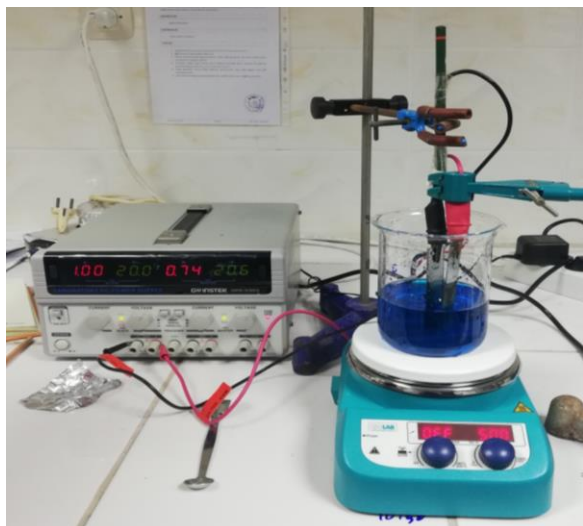
Fig. 2. Experimental set-up for the electro-Fenton oxidation process
