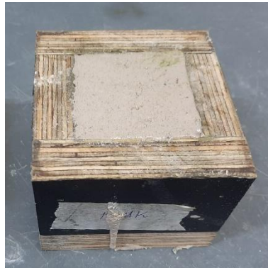
Fig. 3. 50*50*50 mm metakaolin-based geopolymer mortar sample
