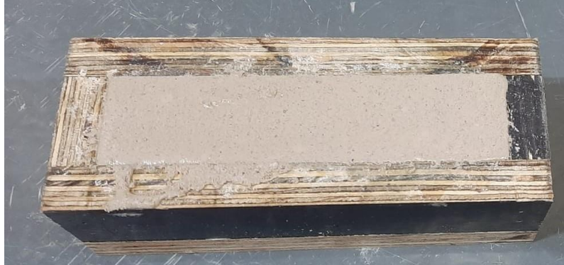
Fig. 4. 40*40*160 mm metakaolin-based geopolymer mortar sample
