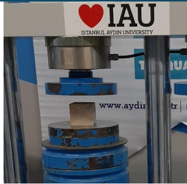
Fig. 6. Compressive strength test conducted on metakaolin-based geopolymer mortar
