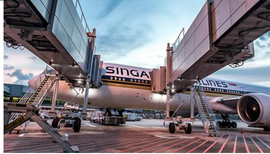
Figure 1. Passenger boarding bridge.
