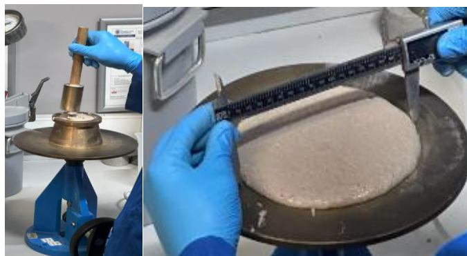
Fig. 5. Mini-slump test conducted on metakaolin-based geopolymer mortar
