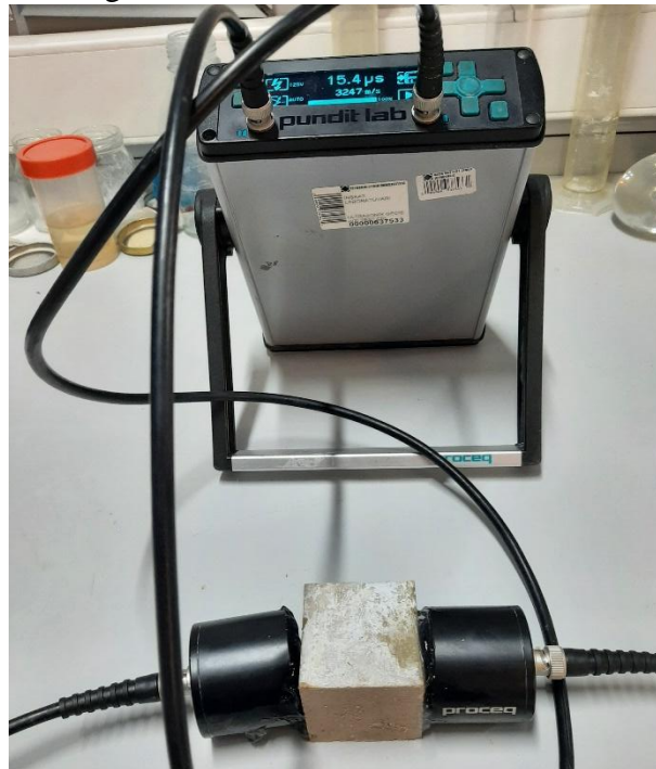
Fig. 7. UPV test conducted on metakaolin-based geopolymer mortar
