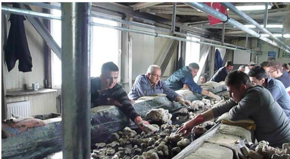
Figure.3. Hand sorting in Bigadic Borate Concentrator Plant Turkey, (Strauss. 2016).
