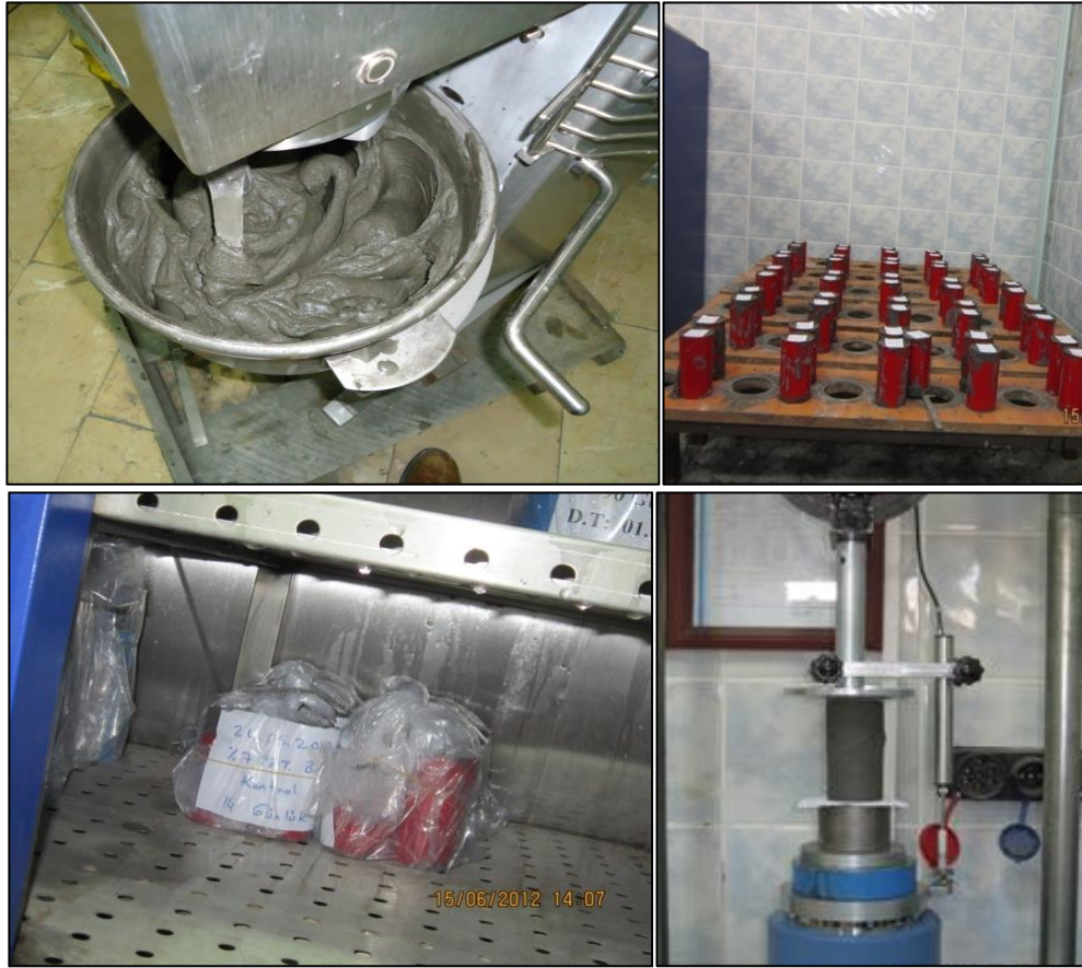
Figure 2.2. Sample casting, curing processes and compressive strength in paste backfilling (Külekçi, 2013)
