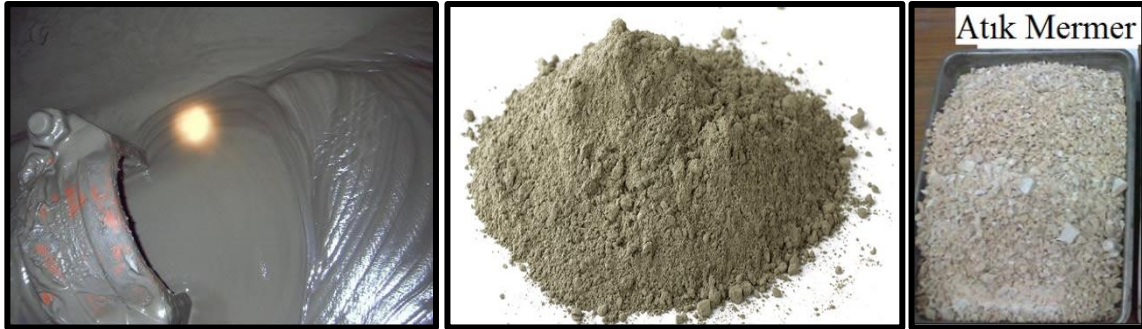
Figure 2.1. Materials used in the study (facility waste,cement/ binder, marble waste)(Külekçi, 2013)
