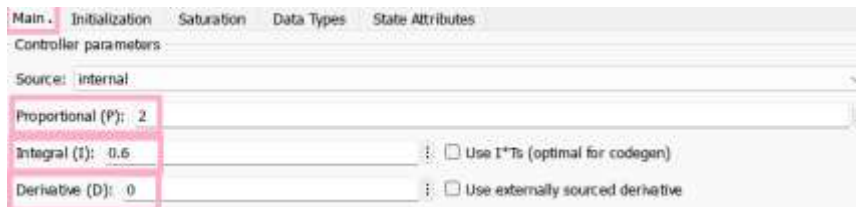
Fig. 8. Adjusting the PID controller main values settings
