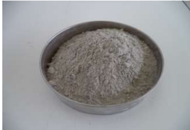
Figure 1: Ground glass powder – fineness \leq 90 \mu\text{m} in diameter
