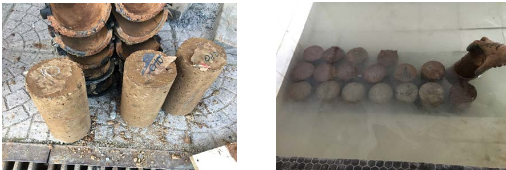
Figure 5. Sampling and curing of concrete
