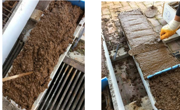
Figure 4. Pouring concrete into molds and gauging process
