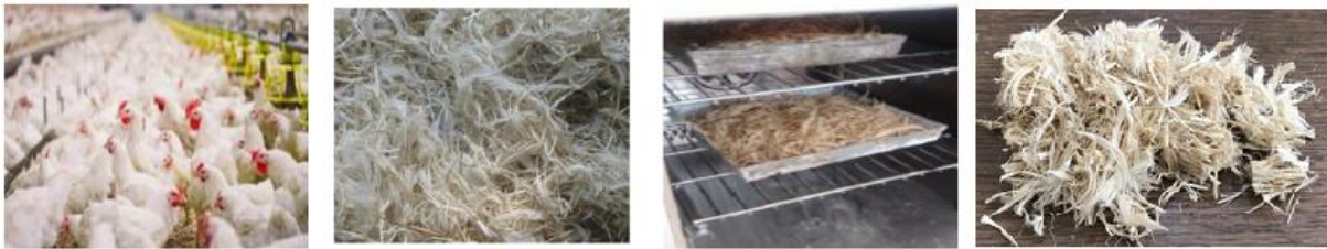
Figure 1. (a) poultry (b) washed waste chicken feathers (c) Drying process of chicken feathers at 35 °C (d) 4-16mm sample
