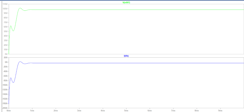
Fig.12. Boost Mode Input Voltage and Current Waveforms
