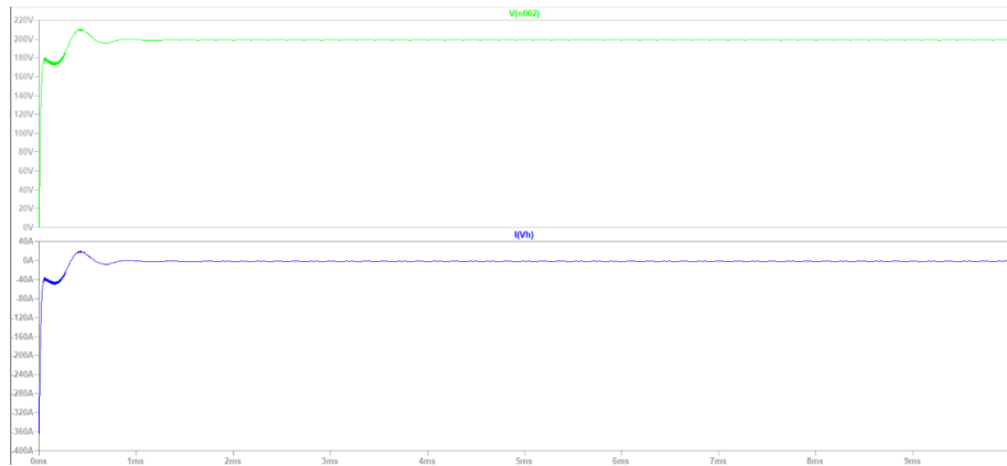
Fig.15 Buck Mode Input Voltage and Current Waveforms
