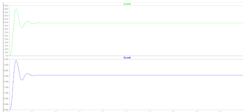
Fig.14 Buck Mode Output Voltage and Current Waveforms
