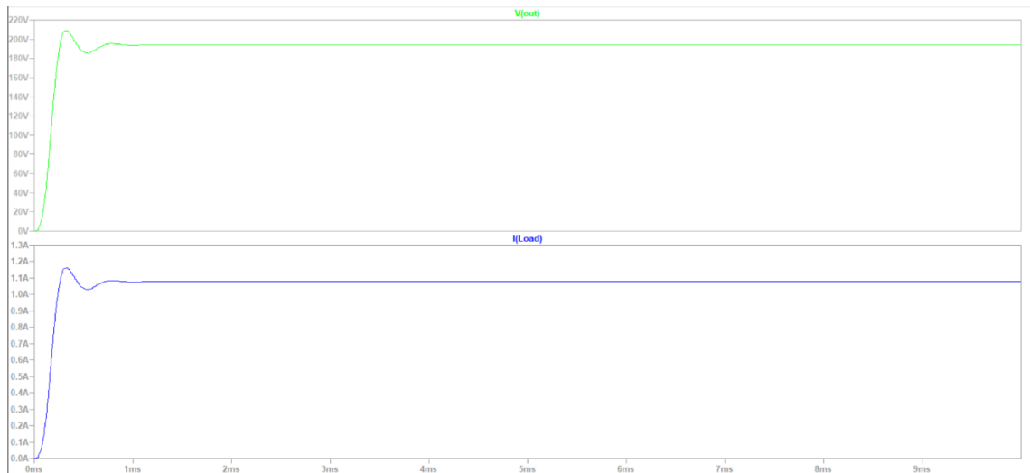
Fig.11. Boost Mode Output Voltage and Current Waveforms
