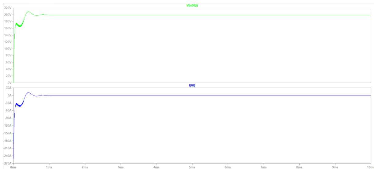
Fig.21 Buck Mode Input Voltage and Current waveforms
