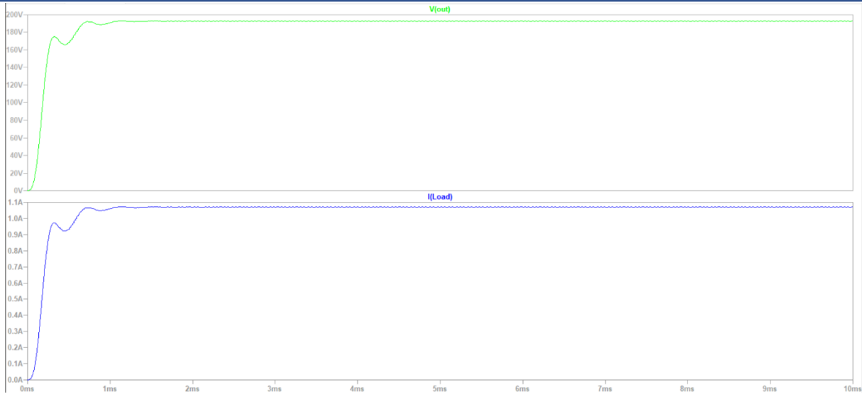
Fig. 17. Boost Mode Output Voltage and Current Waveforms
