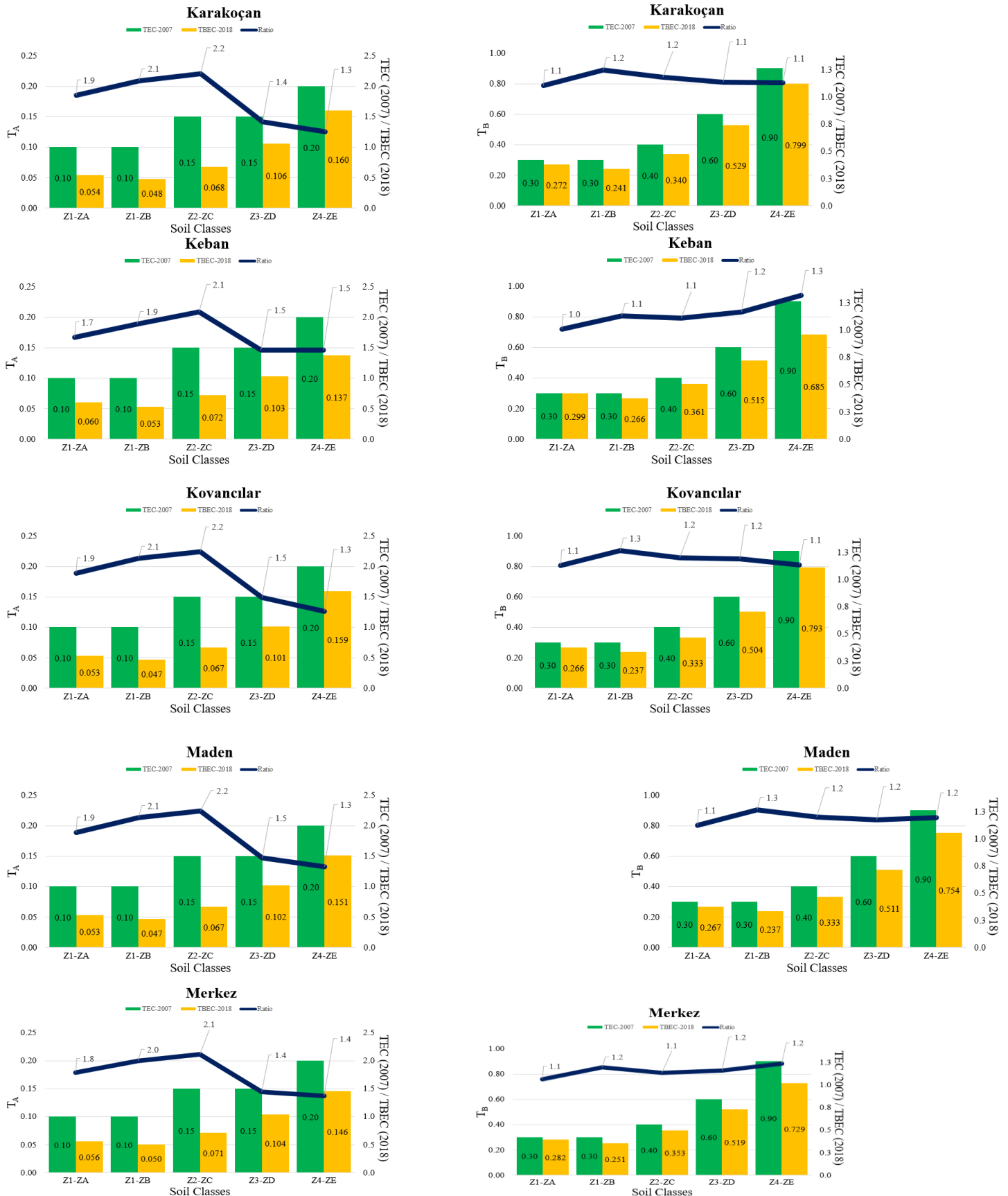
Figure 3.3. Comparison of corner periods for Karakoçan, Keban, Kovancilar, Maden and Merkez districts
