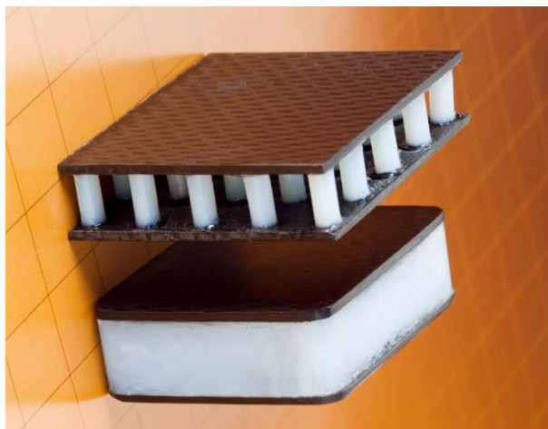
Figure 1. NASA developed ways of creating aerogels that are polymer-reinforced. These aerogels are stronger and can be translucent. Image credit: NASA (Sands, 2023).
