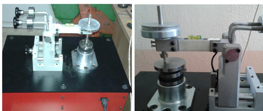
Figure 1. Pin-disc wear system
