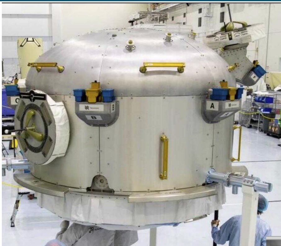
Figure 3. The Nanoracks Bishop Airlock (for ISS) Launch date: December 6, 2020, ( https://en.wikipedia.org/wiki/Nanoracks_Bishop_Airlock ).
