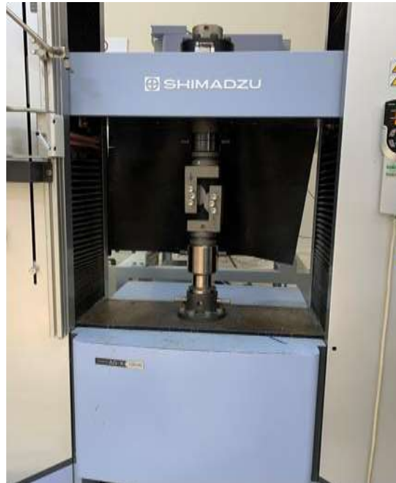
Figure 2.2. Experimental setup for V-notched shear test
