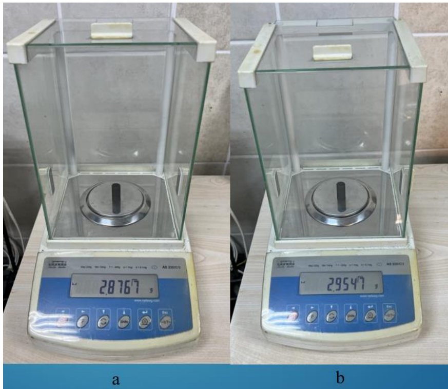
Figure 3. a: Initial weight of the compression specimen; b: Weight measurement after 10 days.
