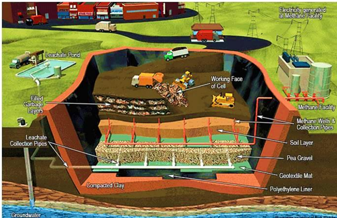
Figure 1: A Typical municipal solid waste landfill system
