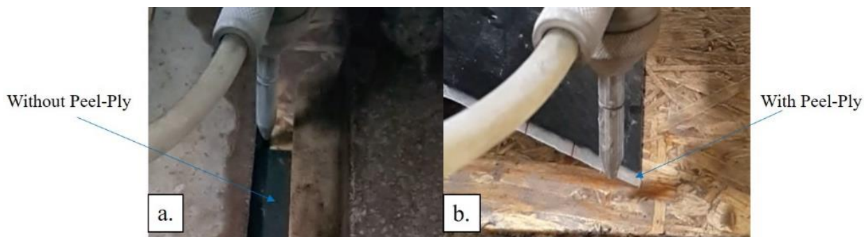
Figure 4. The CFRP Sample Part with Peel-Ply, (b).The CFRP Sample Part without Peel-Ply
