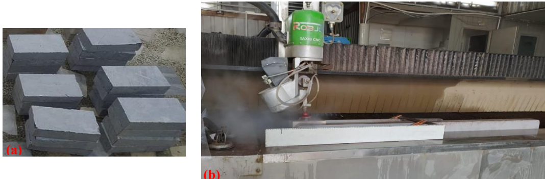
Figure 2.1. a) Dimensioned samples for the experiments, b) Experimental set-up (AWJ cutting machine, enabling the forward angling the jet)
