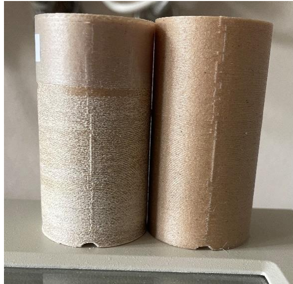
Figure 2. Surface-Activated and Raw Filters; A)Raw Plawood, B)Surface-Activated Plawood
