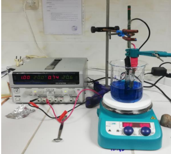
Fig. 2. Experimental set-up for the electro-Fenton oxidation process
