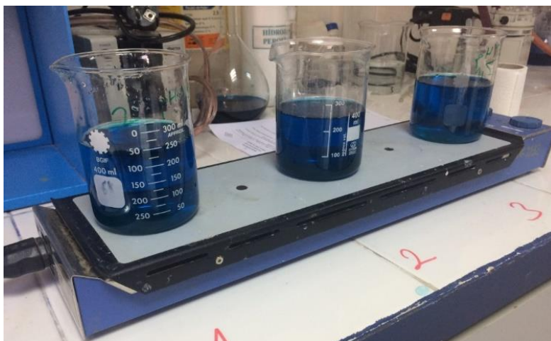
Fig. 1. Experimental set-up for the Fenton oxidation process
