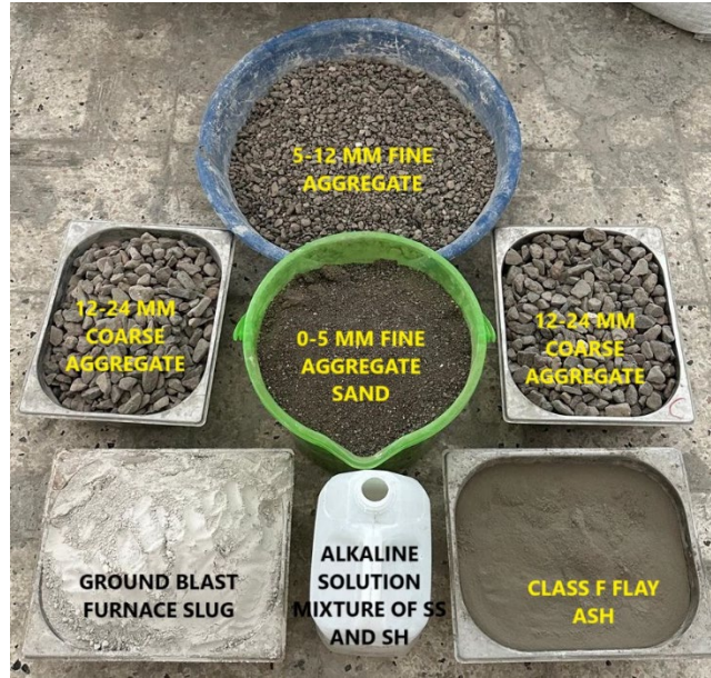
Figure 5: Geopolymer Concrete Components
