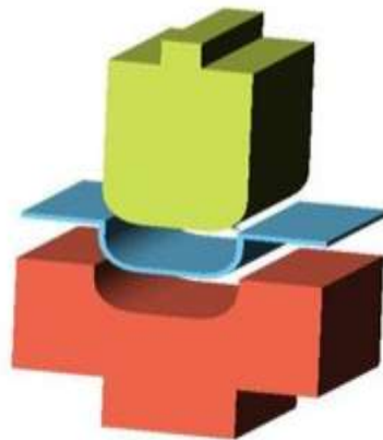
Figure 2. Schematic representation of the bending process (Teknikkutuphane.com 2023)
