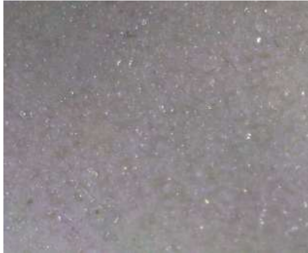
Figure 7. Microscope image (100X) of palm oil and Aerosil 150 reinforced composite according to Experiment 4
