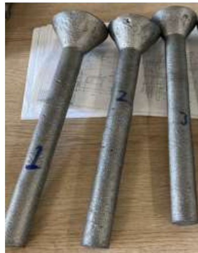
Figure 4. Specimens removed from the sand mold
