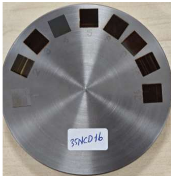
Figure 2.3: Laser induced burns on 35NCD16 low-alloy steel.
