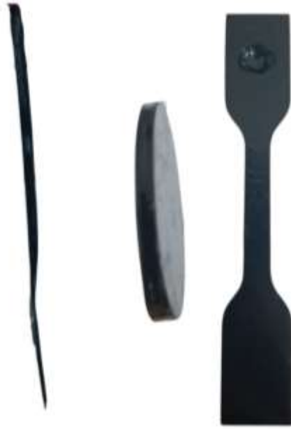
Figure 8. Faulty productions of 1% TiN resin mixture
