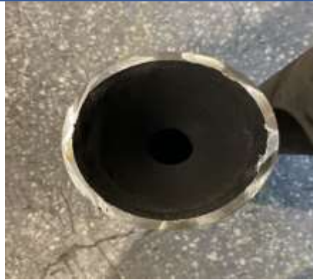
Figure 2: Final state of the sand mold before the casting process
